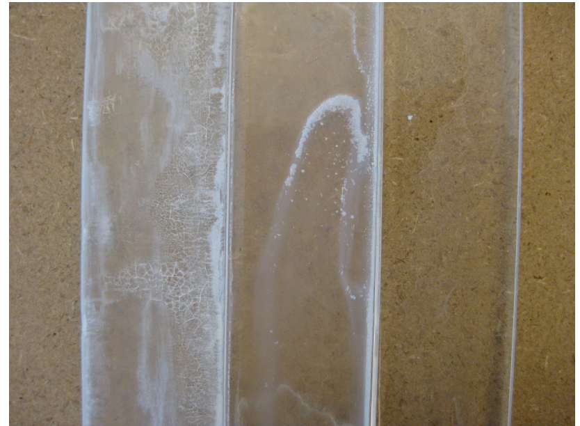
Three lightguides with 3, 2, and 1 coat(s) of 1:3 TPB to polystyrene coating.
