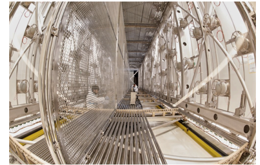
Figure 4: A single module comprising two TPCs.
