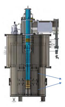
The NbTi coils are impregnated in epoxy to prevent them from moving during when the magnet is energized
