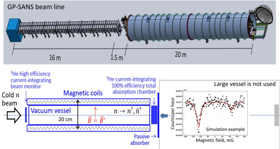
Detailed scan in the range of mag. field  $\pm 1.0$  Gauss with resolution few mG. For 10 days beam time sensitivity reach  $\tau_{nn'} > 24 \ s \ @95\%$  CL. (Detecting fraction~10<sup>-7</sup>)
