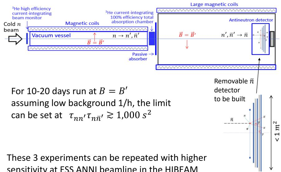
sensitivity at ESS ANNI beamline in the HIBEAM experiment of NNBAR Collaboration
