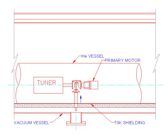
• A gear box with bevel gears is provided between the primary motor and the tuner.
