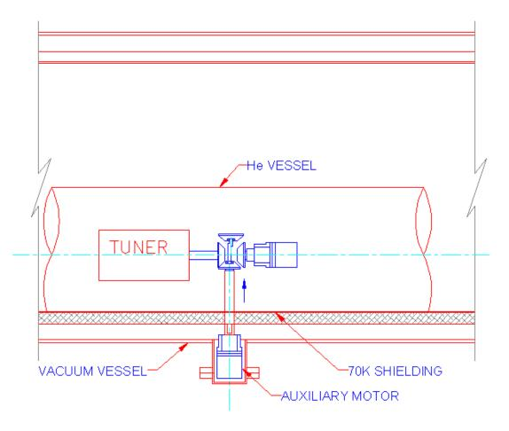
•An inverted cup type structure is fixed on the port. This will carry the motor and provide it rigidity to take the reaction torque.
