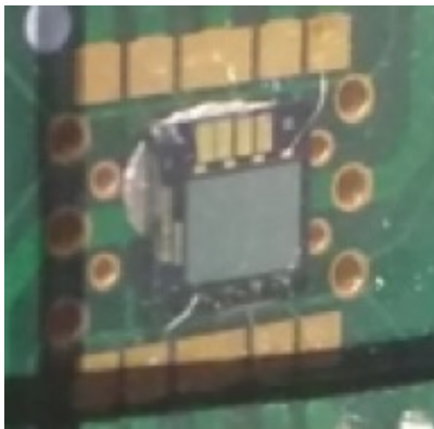
Photo of a 4x4 mm 2 GaInP Photosensor consisting of 10 arrays of 0.5 x 1.5mm 2 size and containing 25 \mu m pixels
