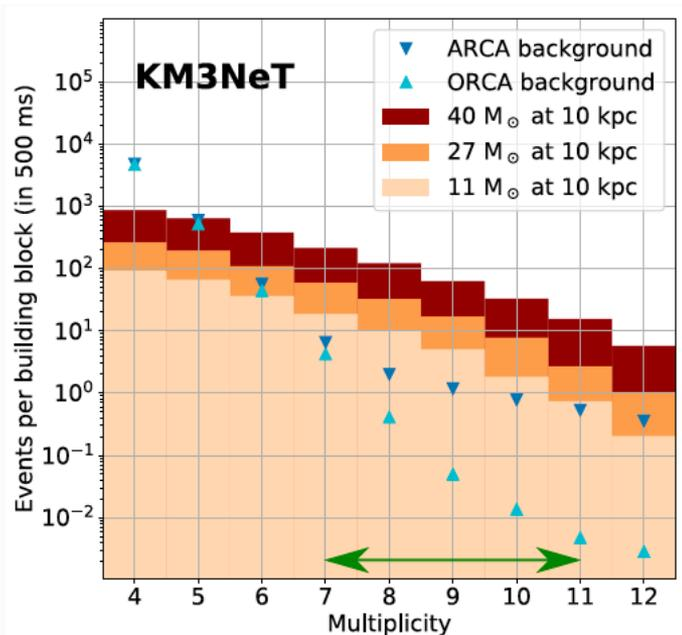
500 ms time window to cover the accretion phase. Expected number of events for signal and background after muon rejection in one KM3NeT building block.
