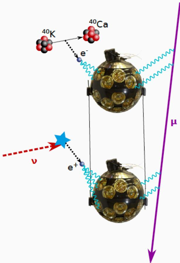
CCSN  $\nu$  low-energy interactions, small tracks of  $\sim 0.5$  cm per MeV; mostly detected as local coincidences on a single DOM. Higher mean energy than radioactive decays.
