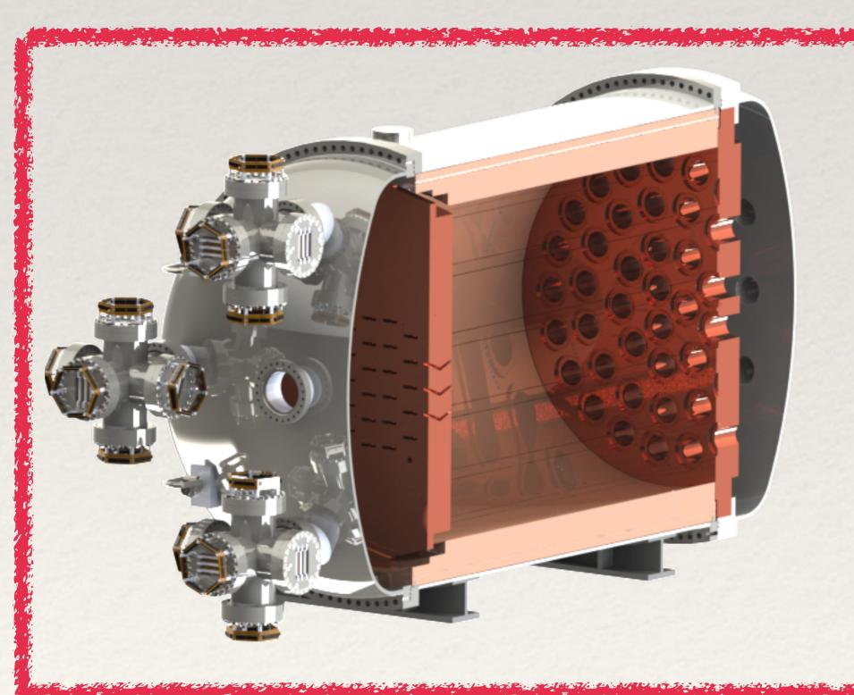
The 100-kg detector is currently under construction and planned to be commissioned during 2022. The energy plane will contain 58 PMTs with 30% coverage and about 3600 SiPMs will constitute the tracking plane.
