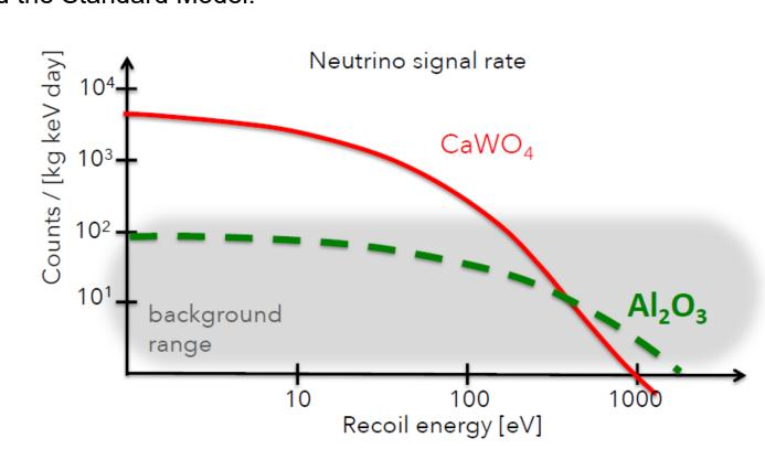
Multi target with CaWO<sub>4</sub> and Al<sub>2</sub>O<sub>3</sub> crystals:
