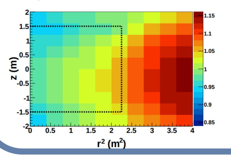
Finally, we correct for the nonlinear response of the scintillator in order to obtain the true deposited energy.
