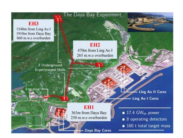
Together, the Daya Bay and Ling Ao I & II nuclear power plants produce 17.6 GW<sub>th</sub>, releasing ~  $10^{21} v_e$  / sec
