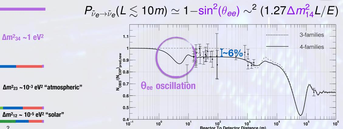
Difficulty in predicting neutrino rate limits the sensitivity of past rate-only measurements, so we need to disentangle the oscillating signature from the absolute rate by getting close to the reactor and measuring the antineutrino spectral shape
