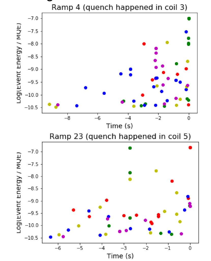
By comparing the "energies" of acoustic signatures with the MQE at the time at which they occurred, we can see how events tend to become stronger relative to the MQE as time passes. However, the nature and strength of this trend is very different for different cases leading to a quench, and there are often "outlier" events which are much stronger than one would expect for a given time. Why such events did not trigger the quench earlier remains unknown.
