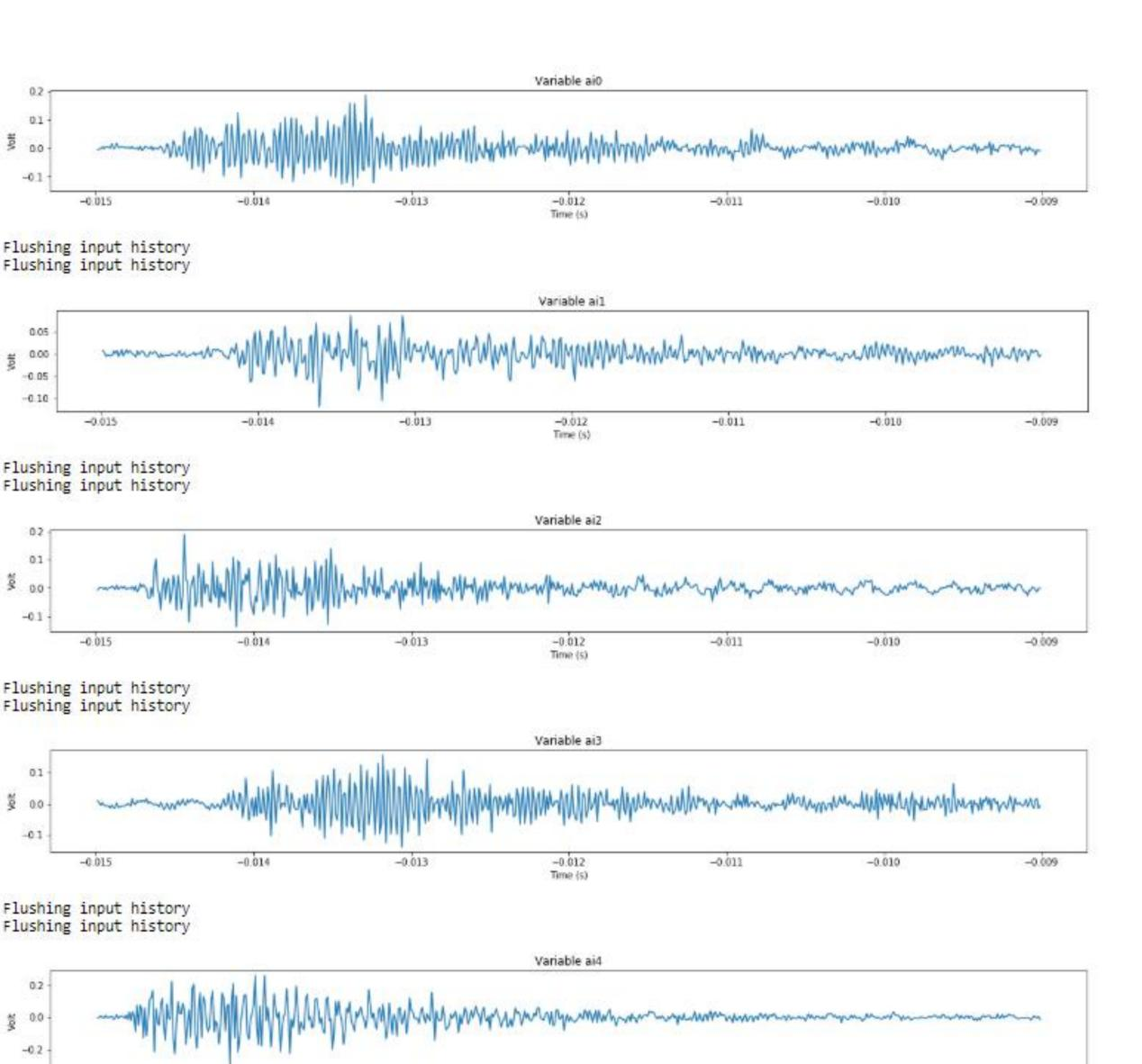
The acoustic events, even we understand (such as those occurring before a just quench), far variability than previously thought in terms of their durations and their relative strengths in the different sensors. This makes it very difficult to develop a useful and consistent notion of the "strength" of an event.
