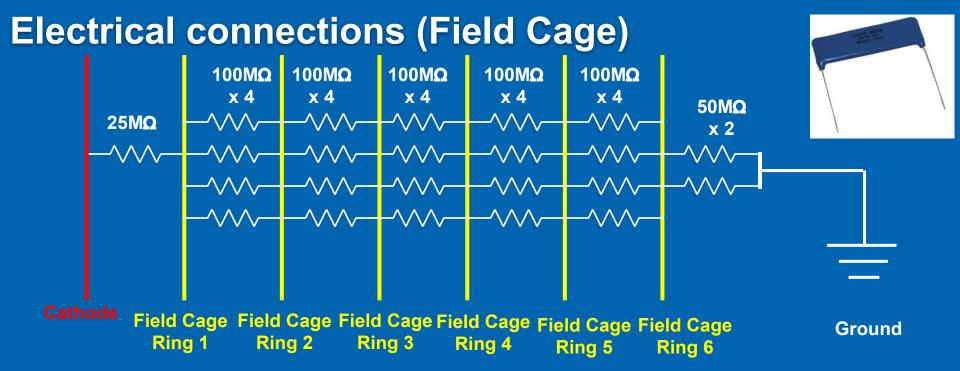
We are going to use two 50MΩ Ohmite thick film resistors mounted externally to the TPC's to provide the last step down to ground and thus leave the last field cage ring at a potential
