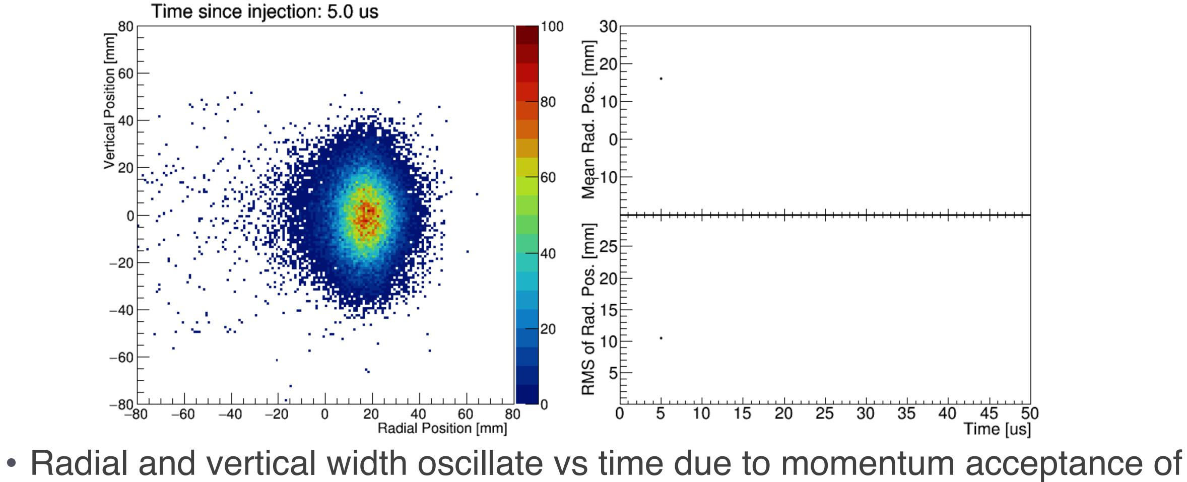
Radial and vertical width oscillate vs beam
