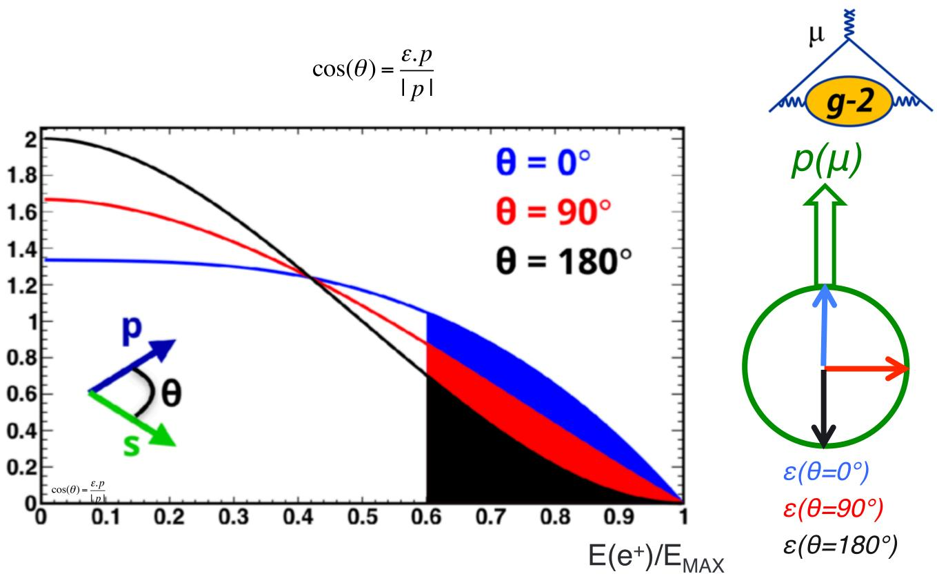
Simply measure the time and energy of decay positrons and count the number above an energy threshold
