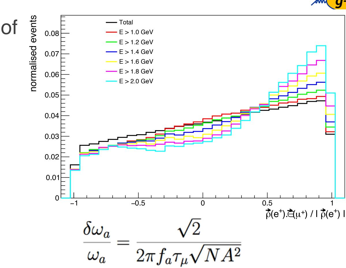
Asymmetry is larger for high momentum e+ Optimal cut at E~1.8 GeV
