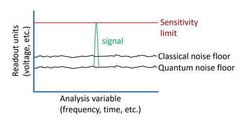
Our approach increases the signal to noise (SNR) by decreasing the noise floor using quantum noise reduction (QNR) and increasing dynamic range using quantum signal modulation
