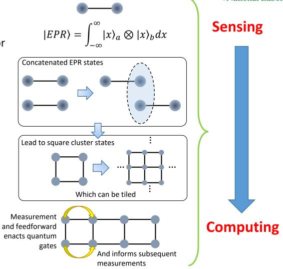
The know-how in generating long range entanglement for quantum sensing lends itself to building quantum computers. This is because in order to make these quantum sensors, one must build a *quantum network* with a *two qubit gate* interaction between the nodes.
