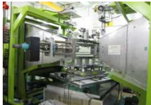
Internal Strain Measurement by Neutron Diffraction at J-PARC
