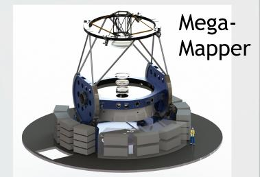
MSE: 11.25m diameter, 1.5 deg<sup>2</sup>, 4332 fibers SpecTel: 11.4m diameter, 5 deg<sup>2</sup>, 15000 fibers MM: 6.5m diameter, 7 deg<sup>2</sup>, 20000 fibers
