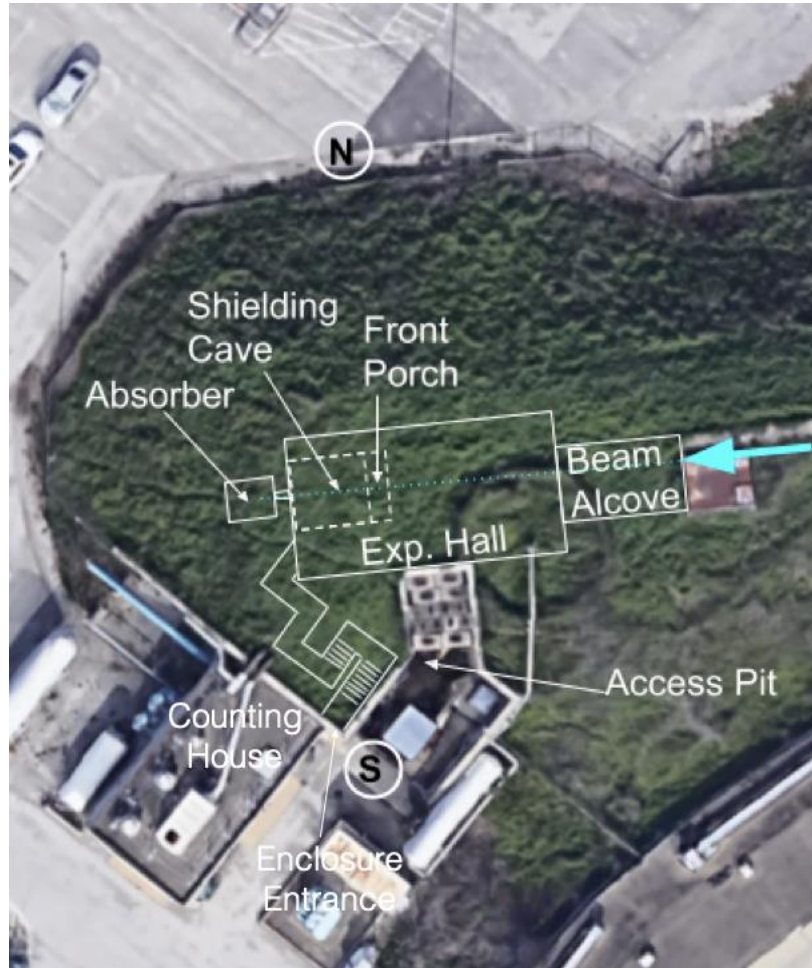
Figure 1: Annotated aerial view showing beam alcove, experiment hall, and counting house approximately as situated in the grass-covered berm. Beam direction and path are indicated by the cyan arrow and dotted line.
