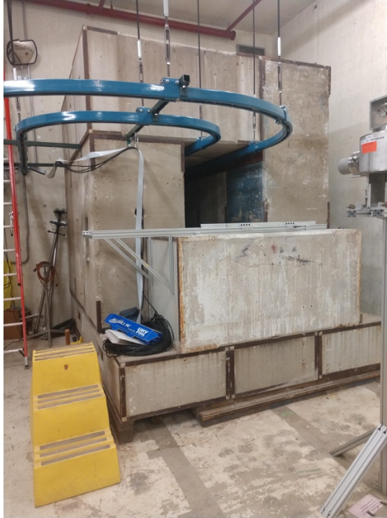
Figure 1: Picture of the experimental shielding cave and front porch block located inside the MTA beam enclosure.
