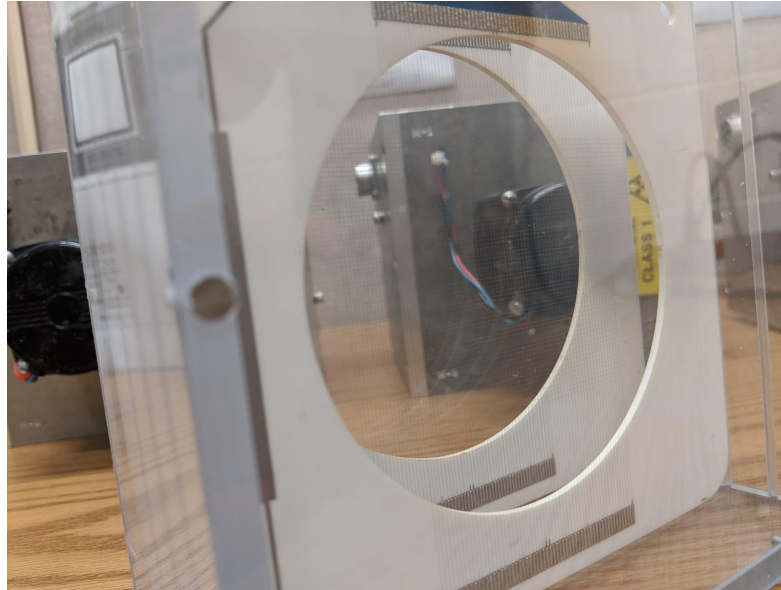
Left: Readout and positioning electronics Center: Close-up of wire planes in ceramic frame
