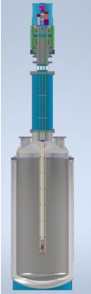
Figure 2: Planned periscope test in a large LAr dewar at LANL as part of QA/QC
