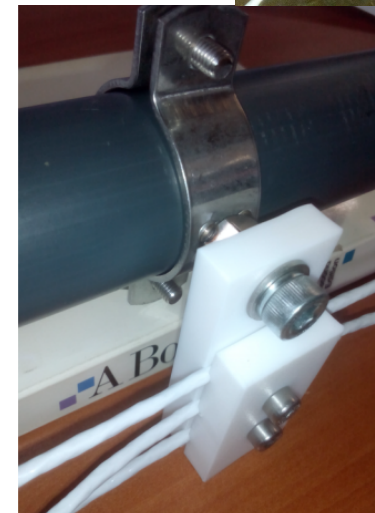
Example cable support On small pipe in ProtoDUNE for temperature sensors from Anselmo Cervera UFIC, Valencia
