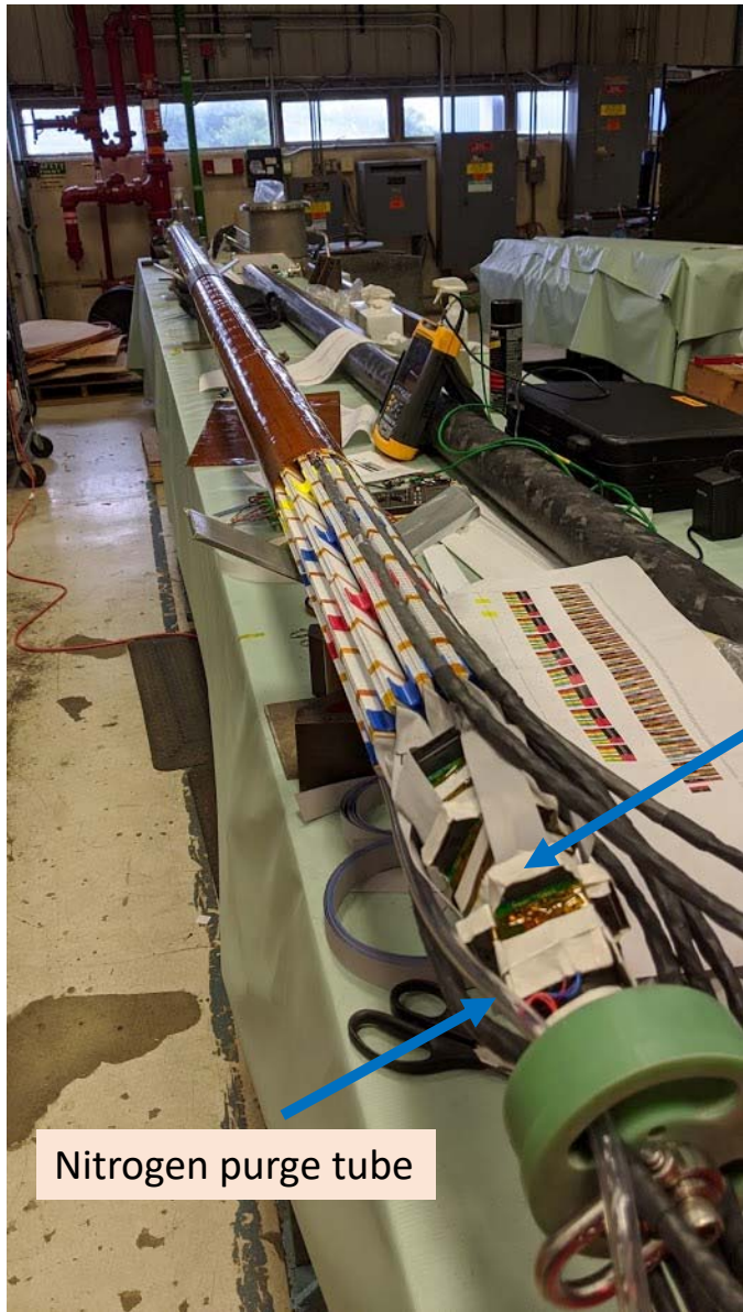
LE interconnect with 1000x gain amplifiers for theta antennas
