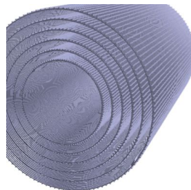
Cylinder design i.e tubes with differing radi - muons still captured but easier for CE to get through.
