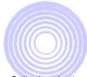
Cylinder design i.e tubes with differing radi - muons still captured but easier for CE to get through.
