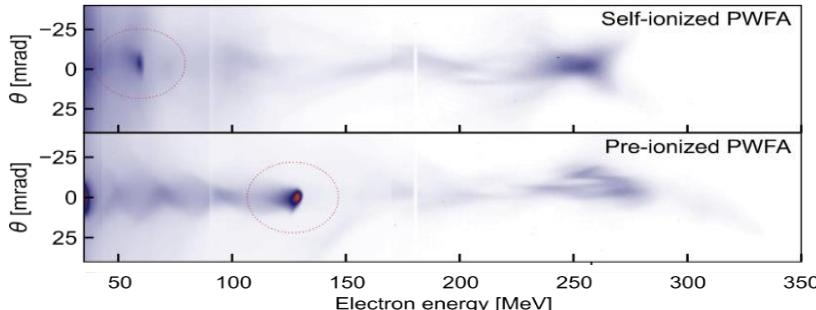
~3.1% total driver-to-witness energy transfer efficiency @ pre-ionized condition
