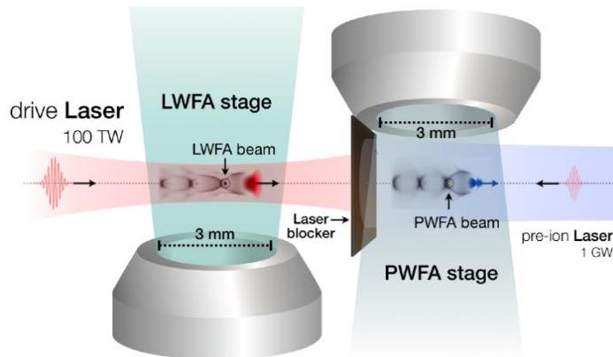
**LPWFA** → Exploiting individual advantages of both plasma acceleration schemes in a truly compact setup for :
