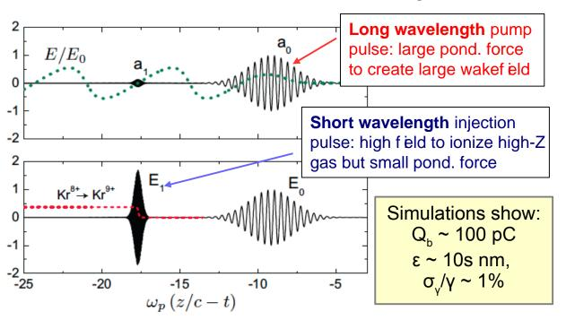
$\rightarrow$   $\epsilon$ ,  $Q_b$ ,  $\sigma_v$  can be controlled via  $a_i$ ,  $w_i$ , + length of high-Z gas  $\rightarrow$  full potential realized with long wavelength drive lasers (e.g.,  $CO_2$  or Tm:YLF), but demonstration with Ti:Sa possible [L. Yu et al., PRL 2014, C.B. Schroeder, PRAB 20154]
