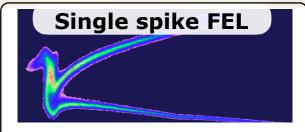
X-ray pulse has single spike when radiation emitted by the electrons in beam tail, travels to beam head in time shorter than few gain times  $\sigma_{z} \sim 0.1 \ \mu m @ 10 \ GeV$
