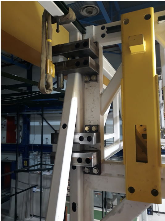
4 hinge blocks mounted to atf.
