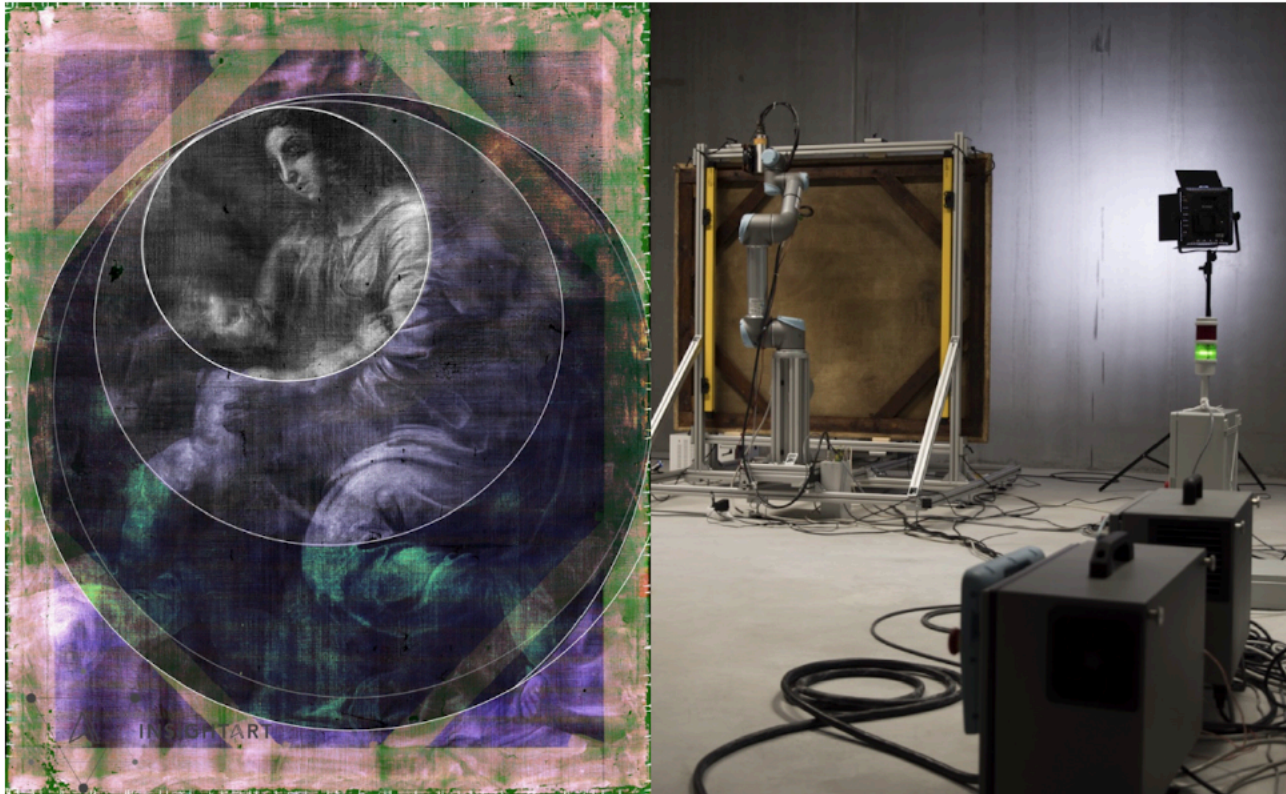
Left: Graphic combining energy spectra measured by RToo scanner (© InsightART, 2019); Right: RToo scanning the painting Madonna and Child (© Jiří Lauterkranc, 2019). (Image: CERN)
