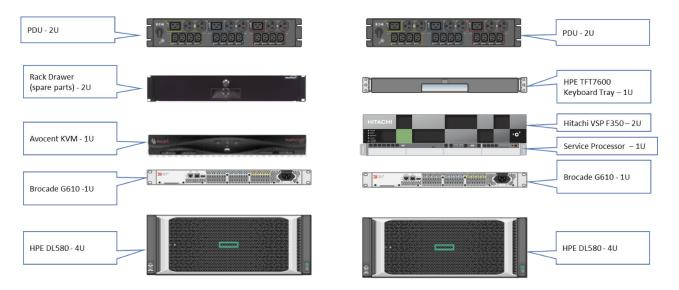
Equipment spread across two racks – total 14U per rack to accommodate cables \* This includes PDU's if they are not already provided.
