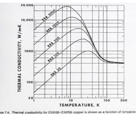
loutated from Equation (7-2) at selected values of the RRR. This figure is adapted from a figure
