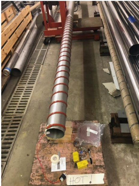
Heat tape wrapped around 6" OD tube in the Fermilab Village.
