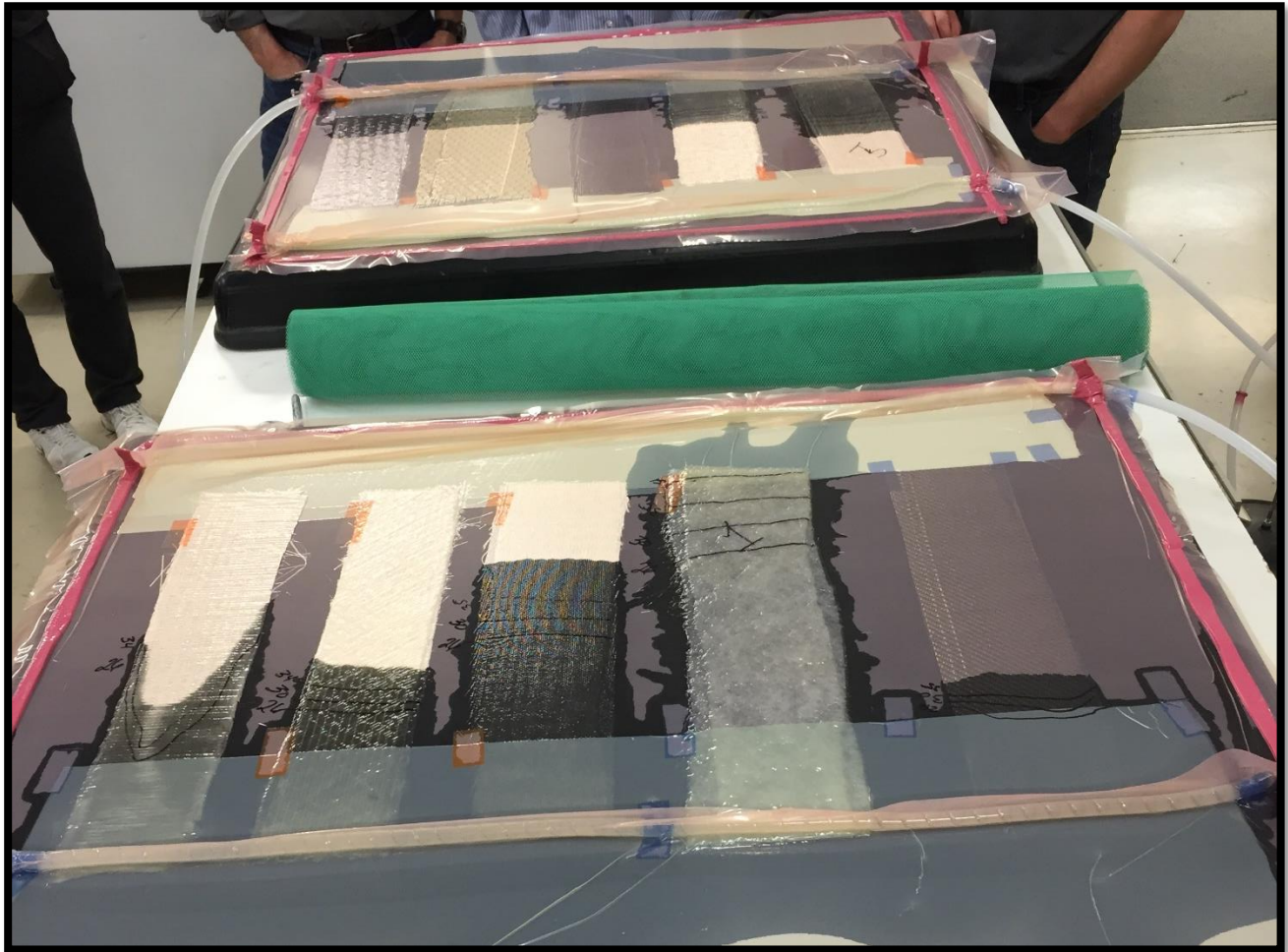
Figure 1. Different RTM test samples showing resin travel over cure time
