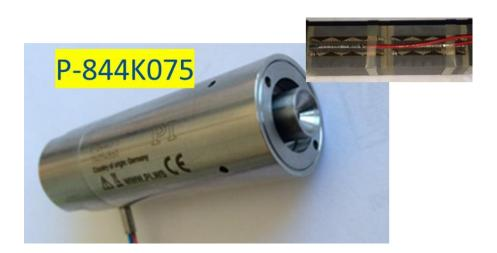
Each capsule has inside two (glued) 10\*10\*18mm PICMA piezos. Piezo, during assembly into capsule, internally preloaded with 800N.
