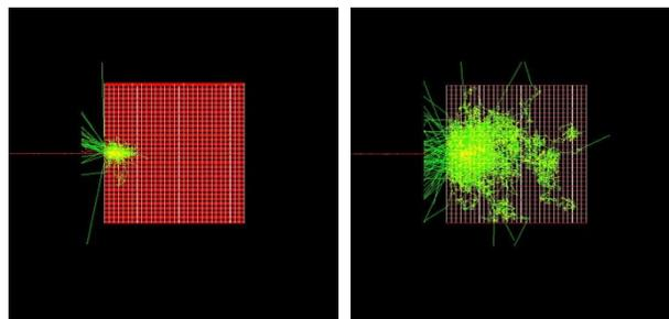
Figure 2. Side view of the development shower of a single event for an electron (left) and a pion (right)
