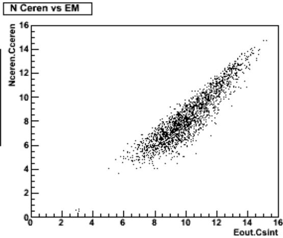
Figure 6. Graph of the corrected values of Cerenkov photons weighted by energy output for 2000 pions at 15 GeV
