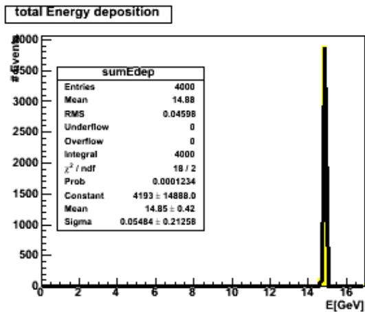
Figure 3. Graph of the total energy deposition. Notice that the mean from the Gaussian is 14.85 GeV
