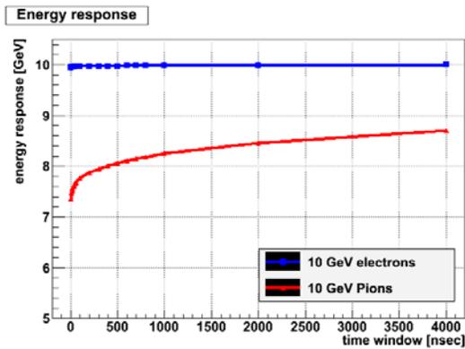
Figure 13. Graph of response for electrons and pions during the first four microseconds
