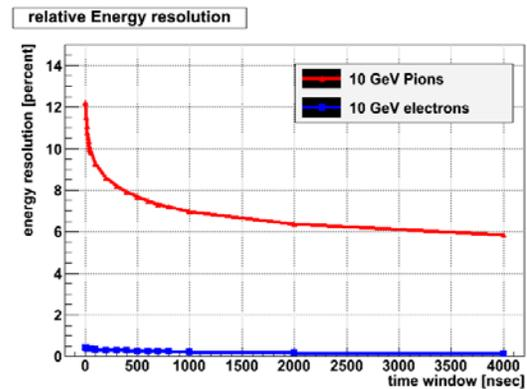
Figure 15. Graph showing resolution for electrons and pions during the first four microseconds
