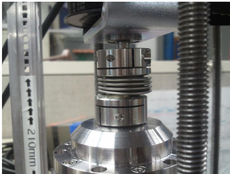
Figure 16 The coupling has broken below the bellow because of misalignment.
