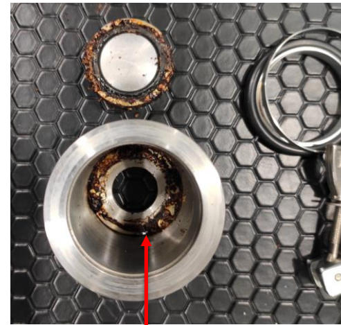
Dirtiness in the overpressure valve for practice coil CR120
