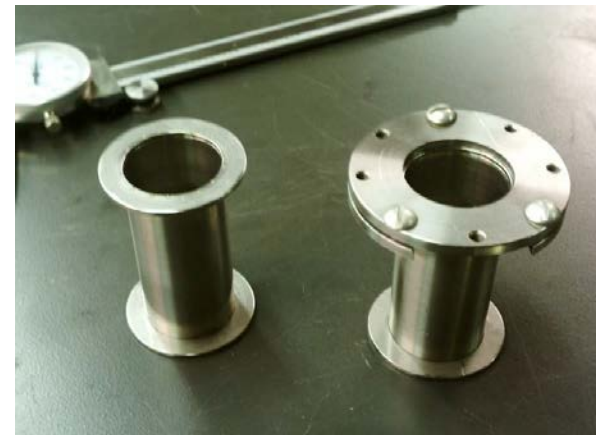
S.S. Dummy (4" high, 1.5" dia.)
