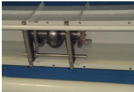
Single cell TE1CAT001 mounted on CBP machine
