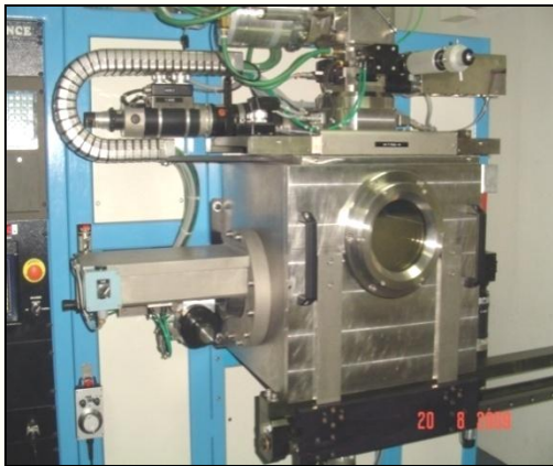
EBW Machine : 6 KW, 60 kV, 450 x 450 x 500 mm chamber size, Vacuum < 5 x 10e-05 m-bar M/s Laxmi Technology & Engineering Industry Coimbtour
