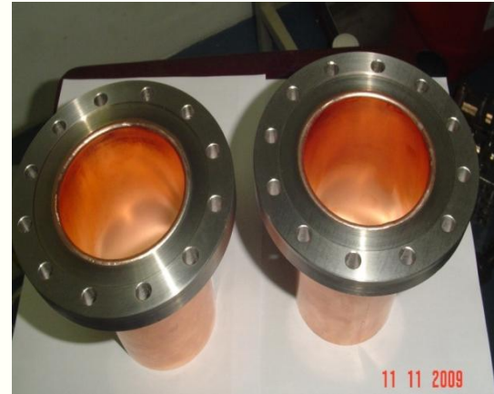
Beam pipe - Flange welding
