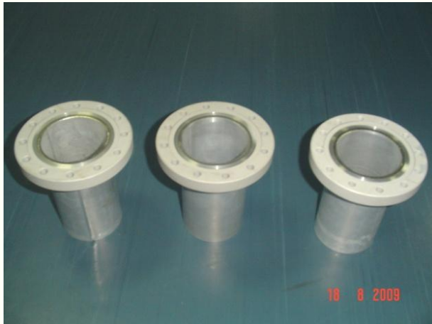
Beam pipe - Flange welding
