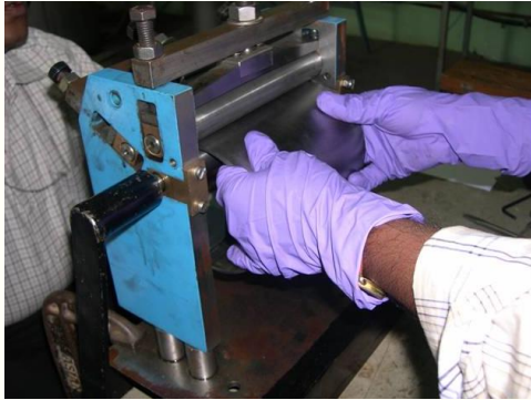
Beam pipe rolling
