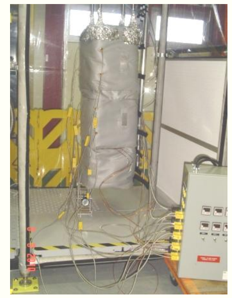
Low temp bake 120 ^{\circ}\text{C} - 48 Hrs @ FNAL
