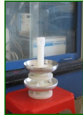
BCP etching fixture with half cells
