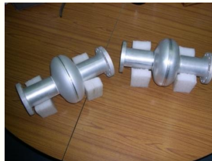
Aluminum and copper Prototype single cell cavities
