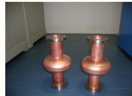
Aluminum and copper Prototype single cell cavities
