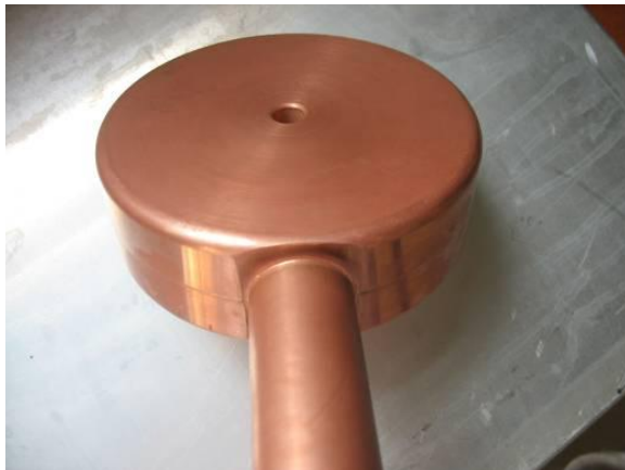
Bulk copper drift tube by electron welding.
