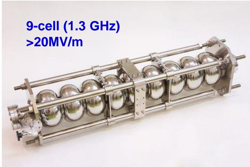
IHEP-01 Low-Loss Large Grain 9-cell Cavity Vertical Test (ILC)
