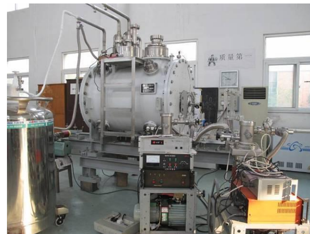
IHEP-01 Low-Loss Large Grain 9-cell Cavity Vertical Test (ILC)
