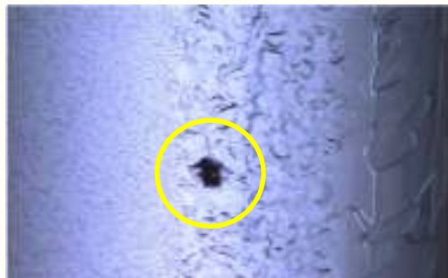
Bump, diameter \sim 200\text{-}300\mu\text{m}
