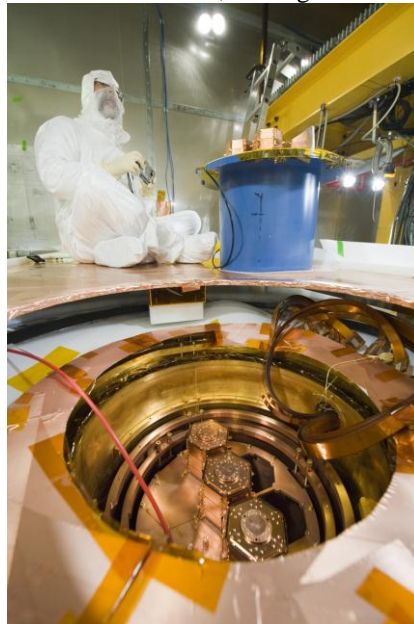
Fermilab scientist Dan Bauer during assembly of CDMS detector system in the cryostat at Soudan mine in Minnesota.
