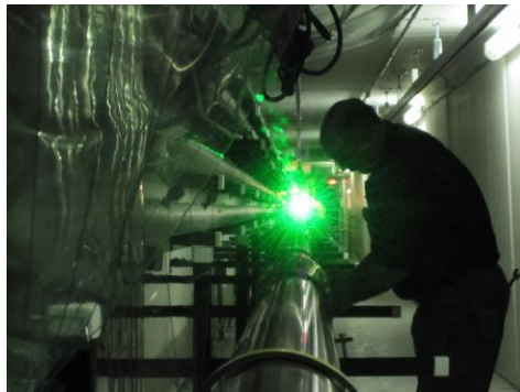
Fermilab scientist James Volk aligns a 40-meter prototype laser cavity for the Fermilab Holometer.
