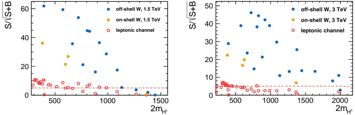
Figure 2. Expected statistical significance for different IDM scenarios,<sup>4</sup> as a function of charged scalar mass, for CLIC running at 1.5 TeV (left) and 3 TeV (right), both for the scenarios with on-shell  $W^\pm$  boson and off-shell (orange)  $W^\pm$  boson (blue). Open red circles show the expected results for the leptonic channel,<sup>2</sup> and the red dotted line denotes the  $5\sigma$  threshold.
