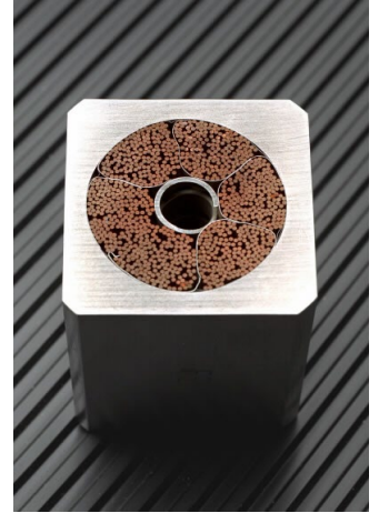
ITER Central Solenoid cable
