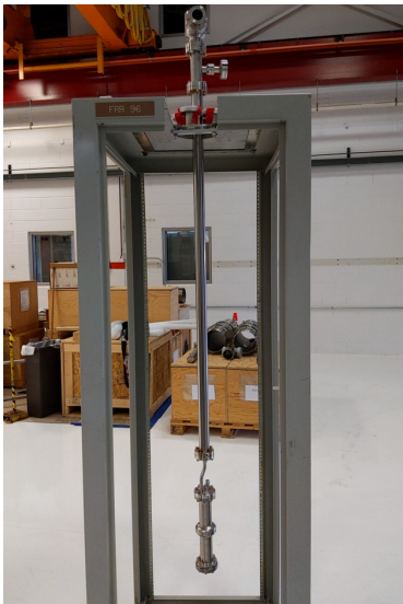
Figure: 3.9 GHz "elliptical" \text{Nb}_3\text{Sn} cavity ready for testing.
