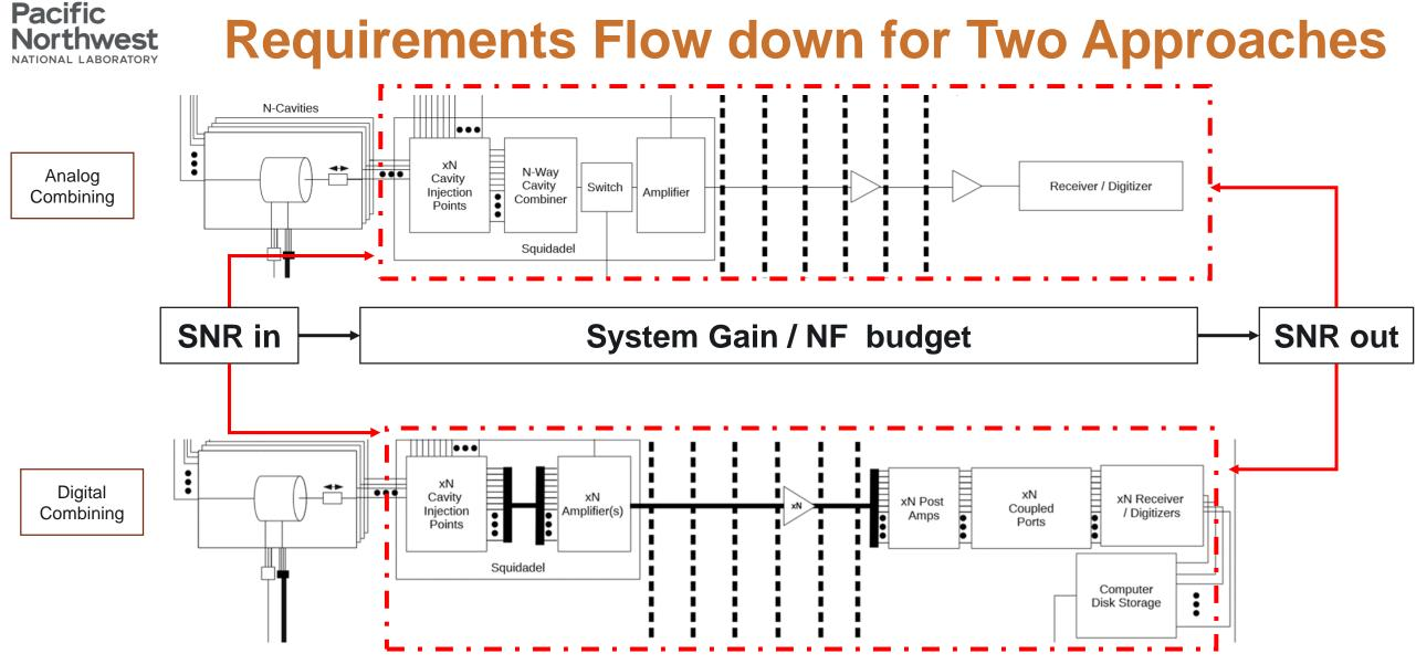
Overall System Noise Temperature requirements will set how much can be allocated to each subsystem regardless of approach.
