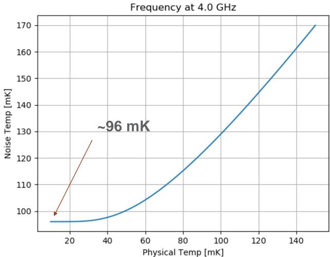
This is the thermal noise model for all the data from this slide onward
