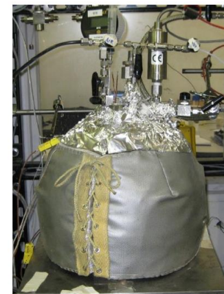
5-L spherical vessel. Experiment done per ASTM E918 standard
