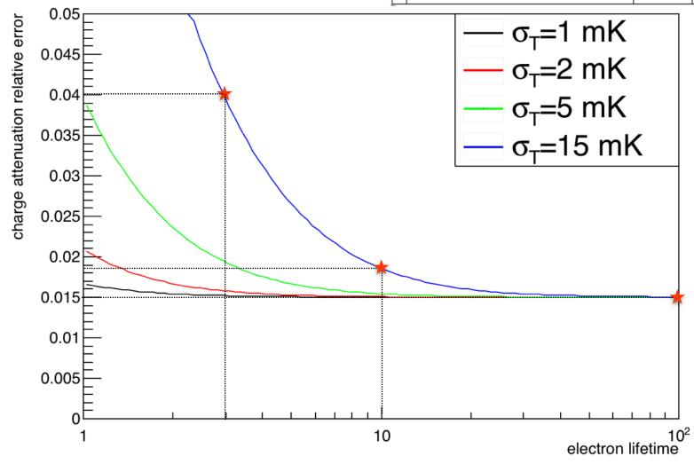
σ<sub>T</sub>=15 mK is equivalent to no temperature measurement and thus to a 5% error on impurity concentration. So we use that curve to compare with Jianming's numbers
