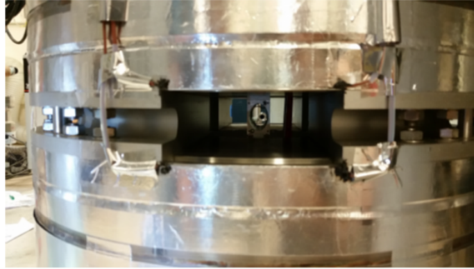
Figure 39: The type-T thermocouple sensors installed on the surface of the magnet reservoir.
