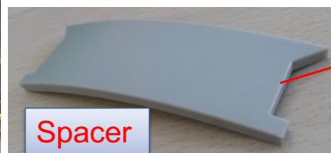
Spoke used as reference for the alignment of the pcb
